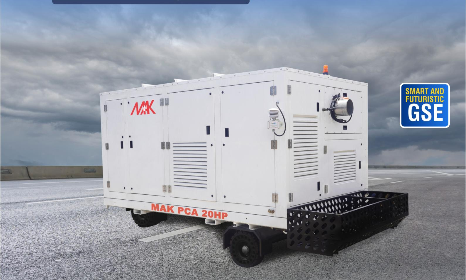
The MAK High pressure preconditioned air unit is designed for cater continuous cooling during ground power-on and maintenance of fighter jet aircraft. It is used to control the heat generation of onboard electronics.
